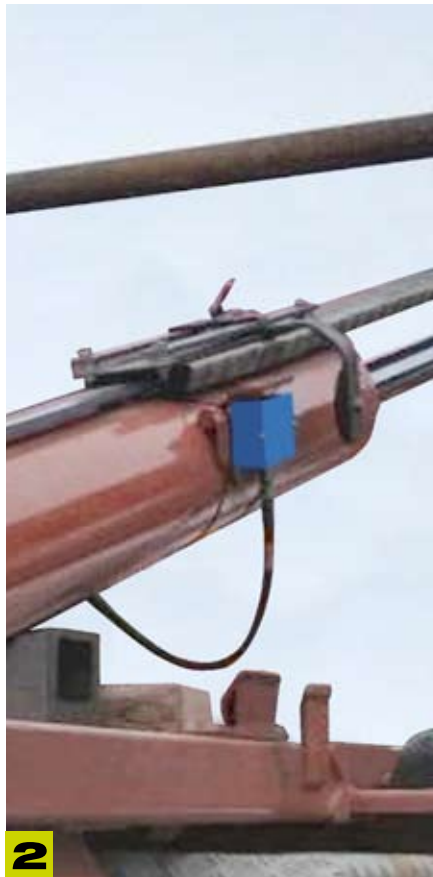
Contactless weighing zone sensor for weight reading
